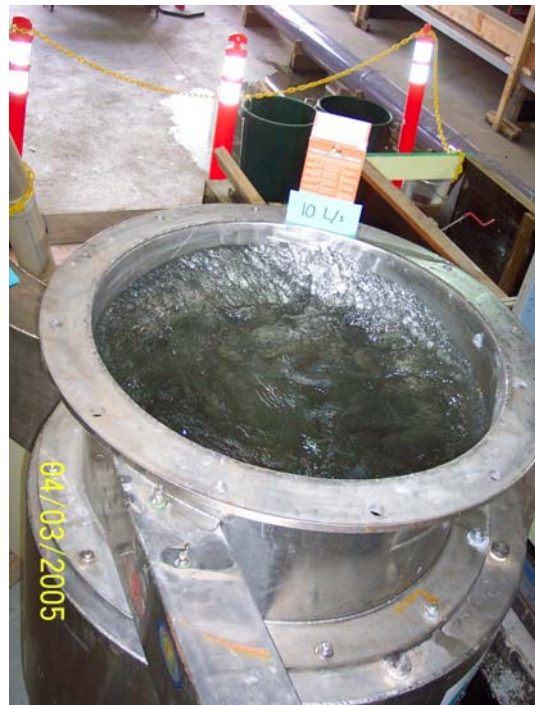
Rapid rotation of water within CDS unit at 10L/s
